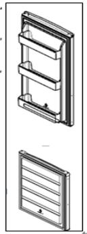
9) Assemble the door of refrigerating
