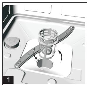
Step 1: contrarotate the Coarse filter ,and then lift it up;
