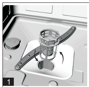
Step 1: contrarotate the Coarse filter ,and then lift it up;
